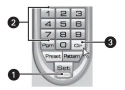
Figure 247. Clearing a Preset Using Web Client
